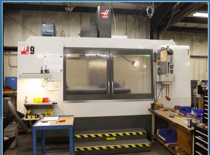
Haas Model VF-9/40 Vertical Machining Center 20 HP 84"x40"x30" w/Wireless Probing System.
