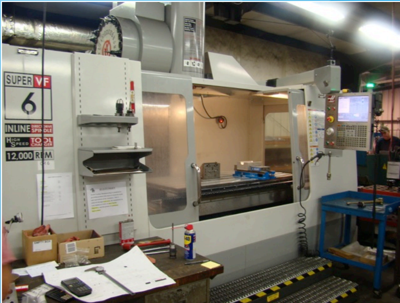
Haas Model VF-6SS Super Speed Vertical Machining Center 30 HP 12,000 RPM Spindle 64"x32"x30" w/Wireless Probing System. HRT310 4 th Axis Rotary Table, TR310 Trunnion 5 th Axis Rotary Table. 4 & 5 Axis Simultaneous Milling
